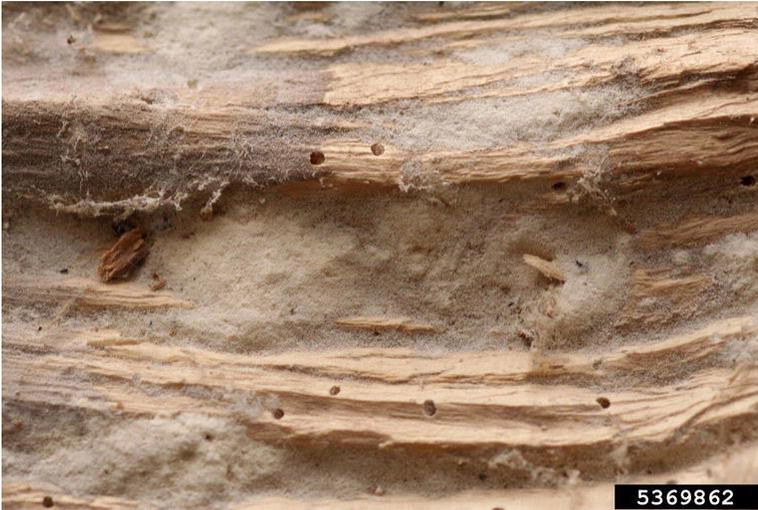
Wood damage from powder post beetles.
